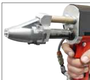
Phase 2 - Blind rivet load
