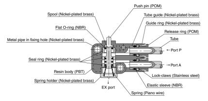
\* Release ring color / Normally closed valve type: Black, Normally open valve type: Light-gray
