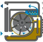
to a continuous film of oil. In this type of compressor no axial thrust is generated so the side surfaces of the rotor are not subject to wear and thus no rotating bearings or thrust bearings are needed. The vanes, too, because of the special way they are
