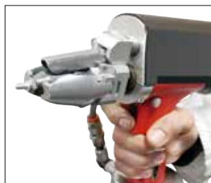
Phase 3 - Blind rivet loaded
