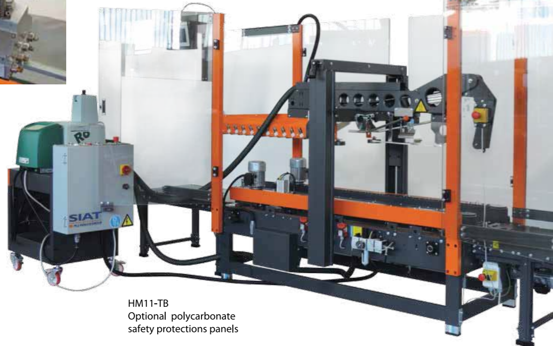
Closing system of the lower flaps (only HM11-TB)
