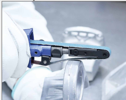
Detail finishing of aluminum material.
