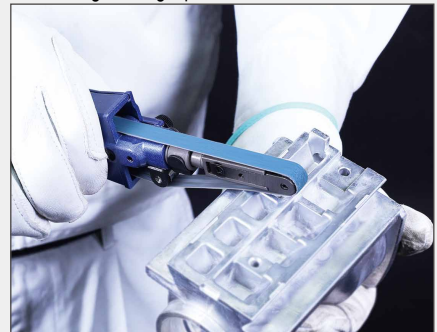
Chamfering of straight parts.
