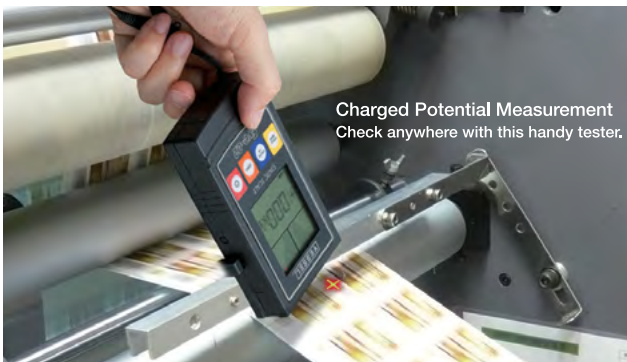
Wide Display The measured potential is displayed with a bar graph and values for quick confirmation
