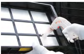
Attach a brush to blow out dust
