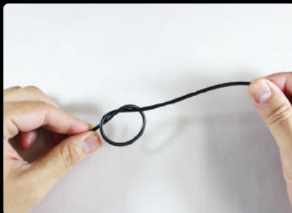
Make a loop at the end of the wire. to prevent tubing from falling off.
