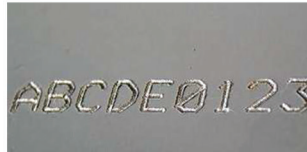
Deep marking on painted steel
