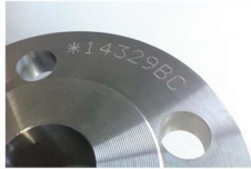
Serial numbering on steel part
