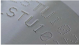
Marking with different dot space
