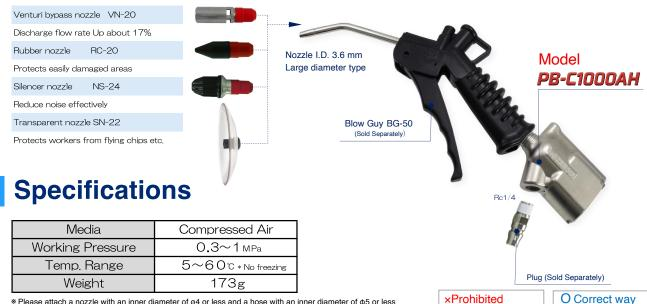
\* Please attach a nozzle with an inner diameter of ø4 or less and a hose with an inner diameter of φ5 or less to the output port. As a guide for the inner diameter of the piping on the supply port side, when using our blow gun, the hose inner diameter is 6.5 mm. When using a nozzle with an inner diameter of 4 mm, please use a hose with an inner diameter of 8 mm or more.
