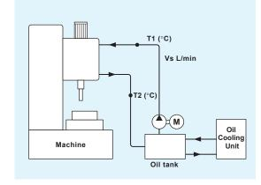
$$Q = \frac{Vs \times \rho \times Cp \times \Delta T}{1000 \times 60}$$
