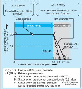
Note: Design the site piping to withstand a pressure of at least 1.0 Mpa.
