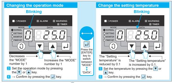
7 To return to the "NORMAL" mode, press the (1) key three times.
