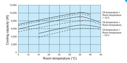
■Solid line —— : When operated at 60 Hz ■Broken line - - - : When operated at 50 Hz
