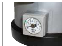
Manometer for air pressure adjustment.
