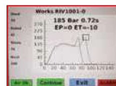
Curve NOK: alarm
