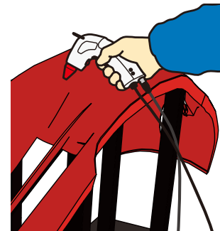
Dust and static-electricity removal from bumpers
