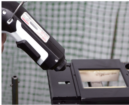
Static electricity removal of resin parts
