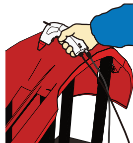
Dust and static-electricity removal from bumpers
